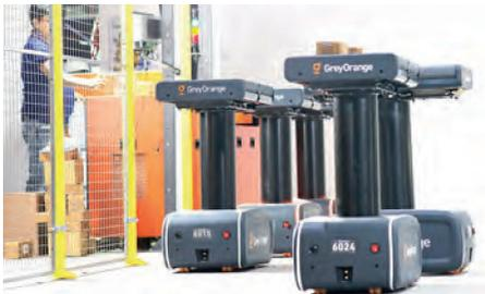
**Above:** The Flexo modular sortation system comprises a fleet of automated robots
