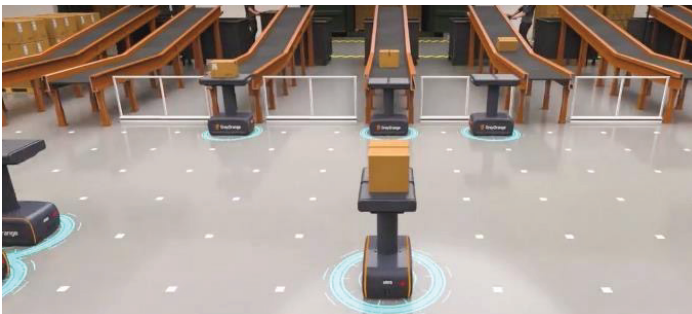
Figure 4: Intelligent movement-based sortation
